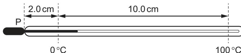
Measuring from P, how long is the liquid column at  $30^\circ\text{C}$ ?
