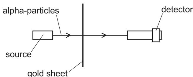
Most alpha-particles pass straight through the thin gold sheet.
